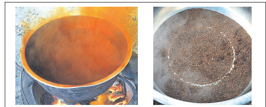
Figure 3. An acrid fumes ( \text{NO}_2 ) produced during refining process.
